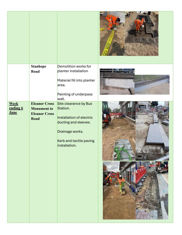
Excavation and preparation for installation of footpath and parking bays.
