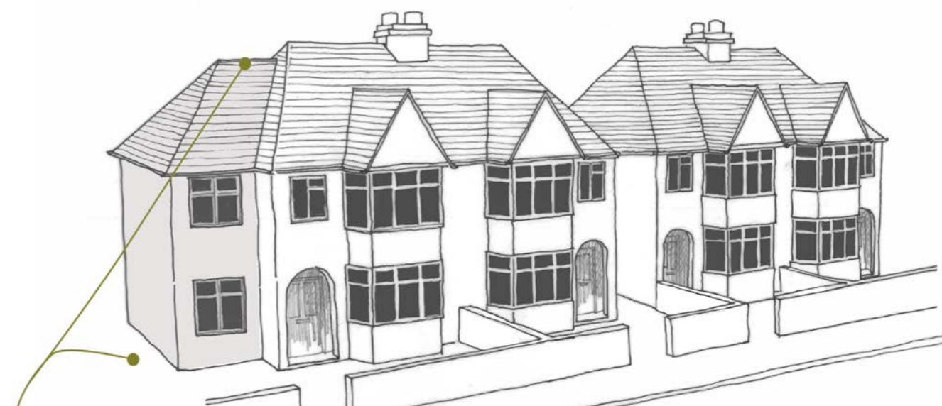
This smaller side extension is more sympathetic to the original façade as it has a reasonable setback from the front façade and the ridge is lower than the original roof thus allowing due prominence to the original house.
