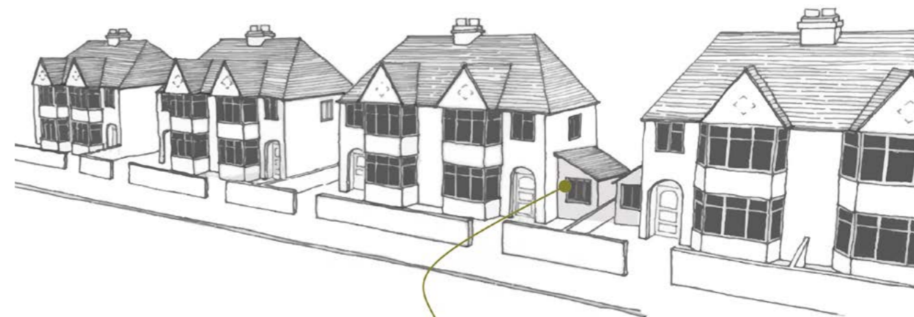
Smaller ground floor only side extensions that are set back from the front façade may be more acceptable in such situations as this helps retain the gap between the houses.
