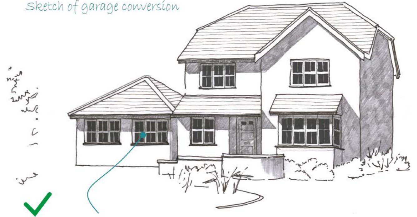
This garage conversion into living accommodation ties in well with the façade style of the house, and would be considered acceptable provided it meets the other design criteria stated in this design guide.
