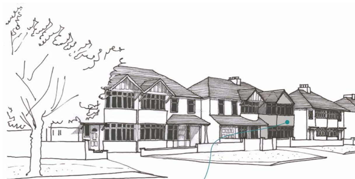
X This double storeyed front extension sits well forward of the other gable features in this row and significantly changes the symmetry of the semi-detached units. This has a negative impact on the streetscene.
